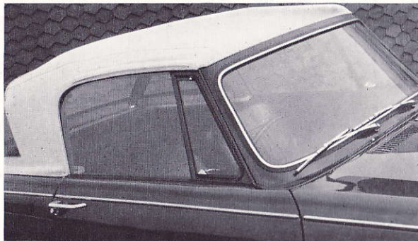
Note the wrap round rear window — part of the Vitesse tradition of excellent visibility. The hood is constructed of tough leather cloth upon a tubular steel frame.
