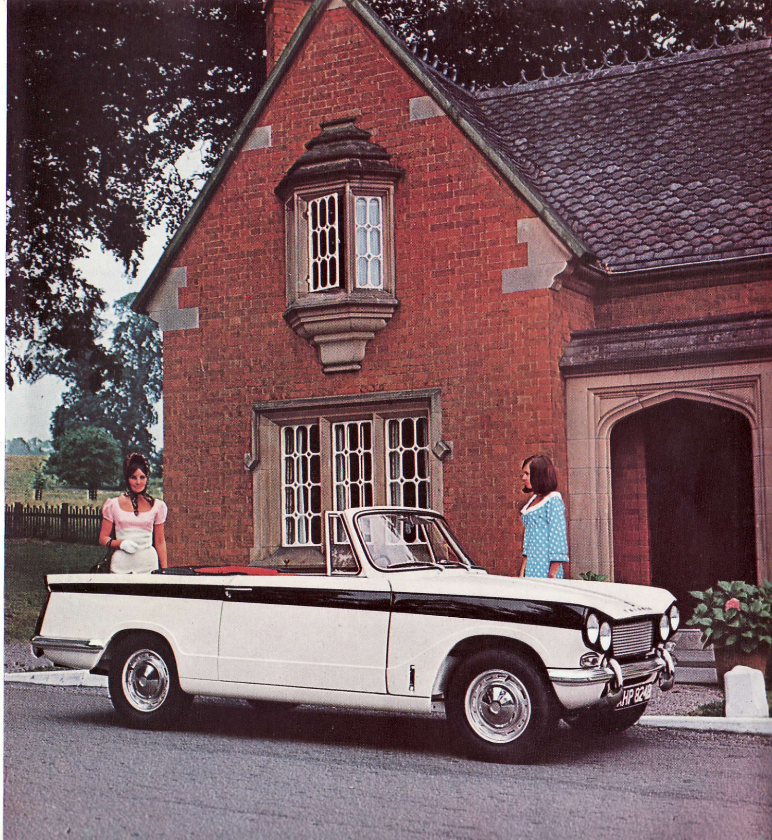
Note the wrap round rear window — part of the Vitesse tradition of excellent visibility. The hood is constructed of tough leather cloth upon a tubular steel frame.
