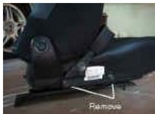
The back of the seat is held to the seat cushion on each side. Start by removing the single Phillips head screw (the '99 has an 8mm nut) with large washer from the hinge point on the side of the seat which does NOT have the seat tilt lever. You can leave the rest of the plastic parts in place for now.
